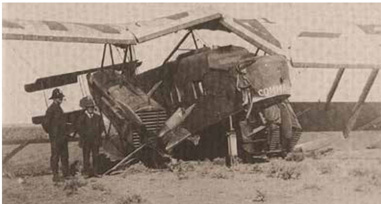
Fig.5: The undercarriage and wings absorbed the impact of the crash landing.(Source: Museum Africa Collection)
