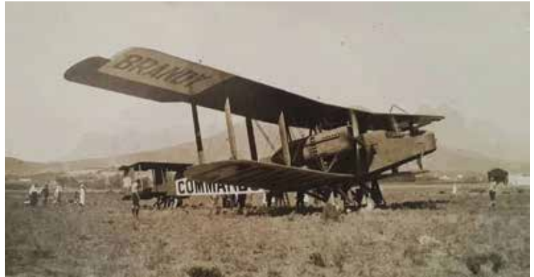
Fig.1: For the time, the Handley Page O/7 was considered an extremely large aircraft that could carry passengers in an enclosed cabin. Note the open seat in the nose. It was suggested this position could be used to drop mail without having to land.
