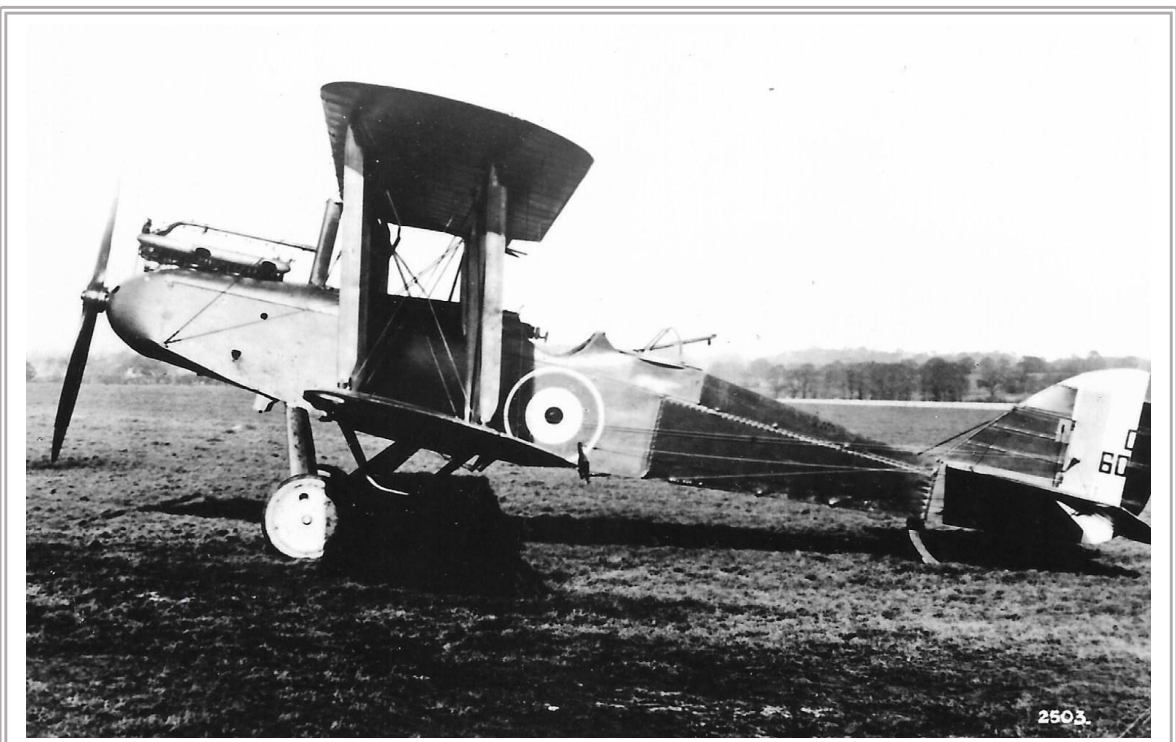
DE HAVILLAND 9 Fitted with one 230 h.p. Siddeley Puma engine
